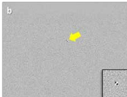
Figure 2. Images collected via a) standard vs. b) enhanced vision of the surface of a bare silicon wafer with one small defect are shown. The insets show magnified views of the defect. The small defect is easily observable in enhanced vision. The larger image dimensions are  $550\ \mu\text{m} \times 413\ \mu\text{m}$ .
