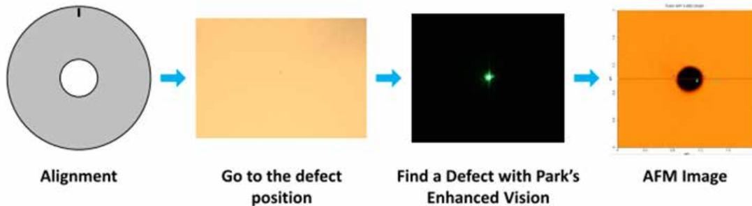
Figure 5. The new ADR-AFM process with newly introduced dark field enhanced vision for hard disk media with reflective surface.
