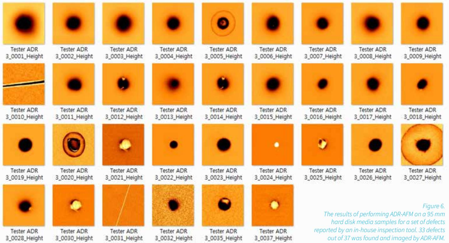
Figure 6. The results of performing ADR-AFM on a 95 mm hard disk media samples for a set of defects reported by an in-house inspection tool. 33 defects out of 37 was found and imaged by ADR-AFM.
