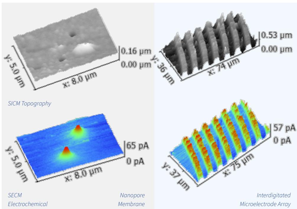
(Bottom) Scanning electrochemical microscopy (SECM) is used to measure diffusion of redox active molecules through the nanopores of the membrane or to measure redox cycling at the microelectrode array.
