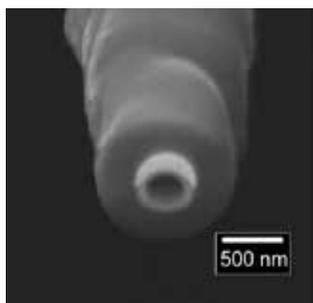
A hybrid scanning electrochemical microscopy – scanning ion conductance microscopy (SECM-SICM) probe. The central barrel is used for SICM and provides distance control, the crescent-shaped gold electrode is used to measure faradaic electron transfer. The entire pipette is insulated in a layer of vapor-deposited parylene.
