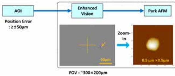
Figure 3. An example of enhanced vision image and how it facilitates linkage between the AOI tool which has larger stage errors and Park ADR-AFM.
