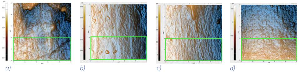
Figure 2 - AFM topography images of the black hair samples: (a) before any prolonged exposure to sunlight; Rq: 4.5 nm, (b) first sample after 42 hours of sunlight, Rq: 4.1 nm, (c) second sample after 42 hours of sunlight, Rq: 4.9 nm, and (d) third sample after 42 hours of sunlight, Rq: 3.1 nm. The green box in Figure 2a is the region in which the Rq value was calculated for that sample; regions of identical dimensions and position were used to calculate the Rq values of the other samples.
