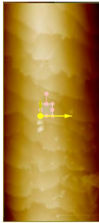
Figure 1a - Example of selecting a  $5\mu\text{m} \times 5\mu\text{m}$  region on a sample hair for surface roughness analysis. Above is a  $40 \times 100 \mu\text{m}$  AFM topography image of black hair after 42 hours of sunlight radiation. A small region on the surface, free of any step or scale edges, has been chosen for roughness measurement.
