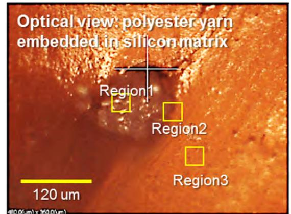
Figure 1: Cross-section of Silicon gel matrix with embedded strand of polyester yarn. Three regions were selected for further investigation: Region 1 on the yarn itself, Region 2 at the interfacial region between the yarn and matrix, and Region 3 on the matrix surrounding the yarn.
