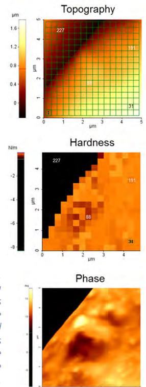
Figure 3. Force-volume mapping array of the sample's interfacial region and the hardness map generated from it. The hardness data correlates to the phase interfacial region.
