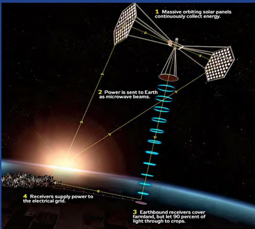
Basic concept of solar energy collected and delivered via satellite and microwave technology. (Illustration: Courtesy Artemis Innovations)
