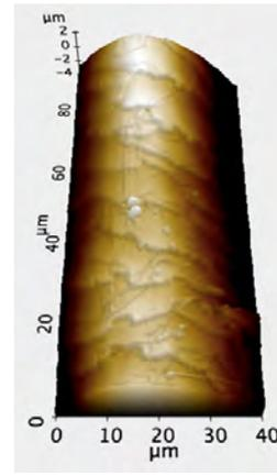
Figure 1b - 3D AFM topography image of the sample in Figure 1a. Because the AFM is able to process Z-directional data by moving the tip up and down, as well as track from side-to-side, such images as above can be produced. 3D renderings of the AFM topography were invaluable in confirming the selected site for roughness measurement was free of step and scale edges.
