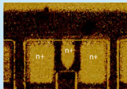
Figure 4. EFM amplitude (top-left), EFM phase (top-right), p-epi ( $2 \times 10^{16} \text{ cm}^{-3}$ ), n well ( $2 \times 10^{17} \text{ cm}^{-3}$ ), p-channel ( $1 \times 10^{17} \text{ cm}^{-3}$ ), n+ contacts ( $2 \times 10^{20} \text{ cm}^{-3}$ ).
