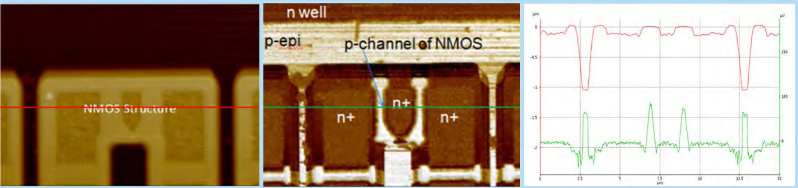
Figure 2. Topography (top-left) and SCM (top-right) data acquired from the sample device. Topography line profile (red line, y-axis on left) and SCM line profile (green, y-axis on right): Doping level: p-epi ( $2 \times 10^{16} \text{ cm}^{-3}$ ), n well ( $2 \times 10^{17} \text{ cm}^{-3}$ ), p channel ( $1 \times 10^{17} \text{ cm}^{-3}$ ), n+ contacts ( $2 \times 10^{20} \text{ cm}^{-3}$ ).
