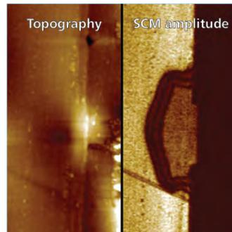
Topography of a FET structure vs. its dopant structure; the brightness in the SCM amplitude image correlates to dopant concentration in this part of the device
