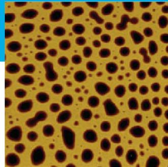
Phase image of lubricant on a plastic board
