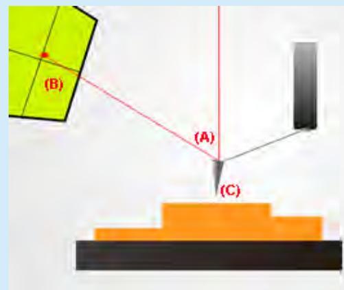
A basic setup for non-contact mode atomic force microscopy. Note the deflected red laser beam (A) shining back up into a sensor (B). This allows the system to keep track of changes in the probe's (C) position. This vertical information along with recorded lateral movements are then combined by software to render an image of the sample's topography.
