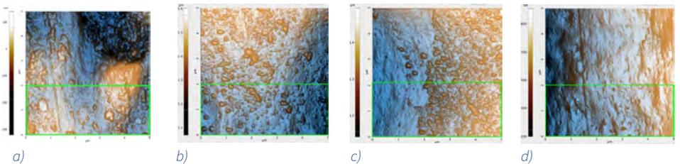
Figure 3 - AFM topography images of the blonde hair samples: (a) before any prolonged exposure to sunlight, Rq: 8.2 nm, (b) first sample after 42 hours of sunlight, Rq: 7.4 nm, (c) second sample after 42 hours of sunlight, Rq: 7.0 nm, and (d) third sample after 42 hours of sunlight, Rq: 4.0 nm. The green box in Figure 3a is the region in which the Rq value was calculated for that sample; regions of identical dimensions and position were used to calculate the Rq values of the other samples.
