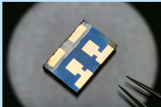
*Perovskite solar cell prototype, These solar cells convert photons to electricity more rapidly than any other material to date, which has gone from just 3 percent in 2009, now predicted to reach up to 31 percent based on new information on how to maximize them.*
